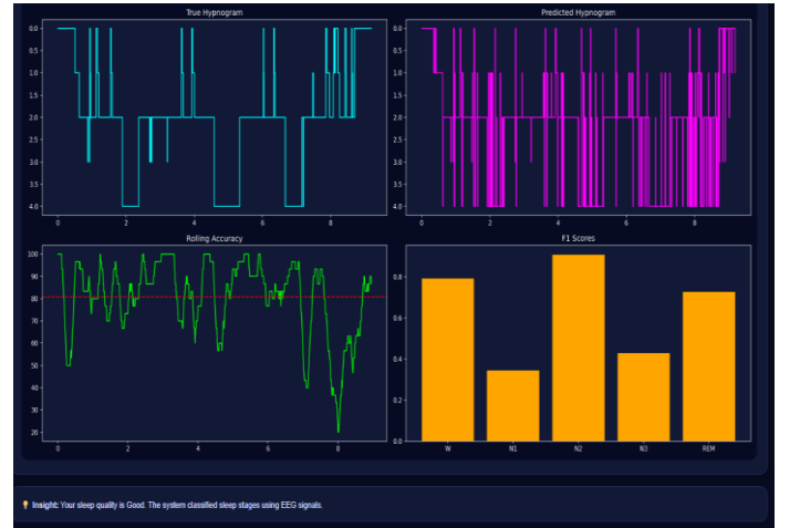
Fig. 4. True vs. predicted hypnograms, rolling accuracy, and per-class F1-scores.
