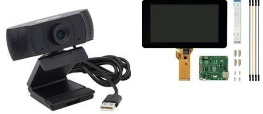
Fig. 5. Peripheral units: (a) the USB camera used for lesion image capture, and (b) the 7-inch HDMI display.
