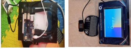
Fig. 7. Implemented hardware: (a) the embedded platform connected to the 7-inch HDMI display, and (b) the assembled prototype unit.
